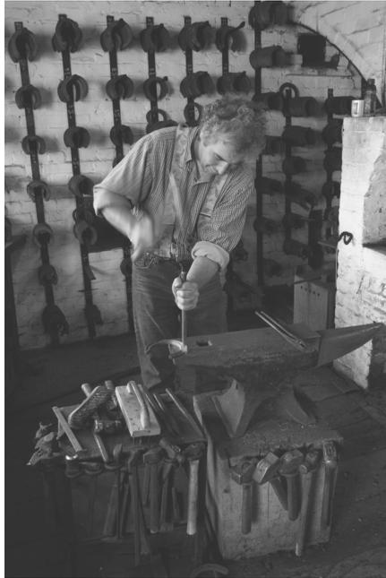
manufacture of horse-shoes has changed little over the centuries. The forge is still fuelled by coke and blasting air through the burning fuel creates the high temperatures required to make the metal red-hot. Today this is done by an electric motor, but in the past bellows would have been used.
